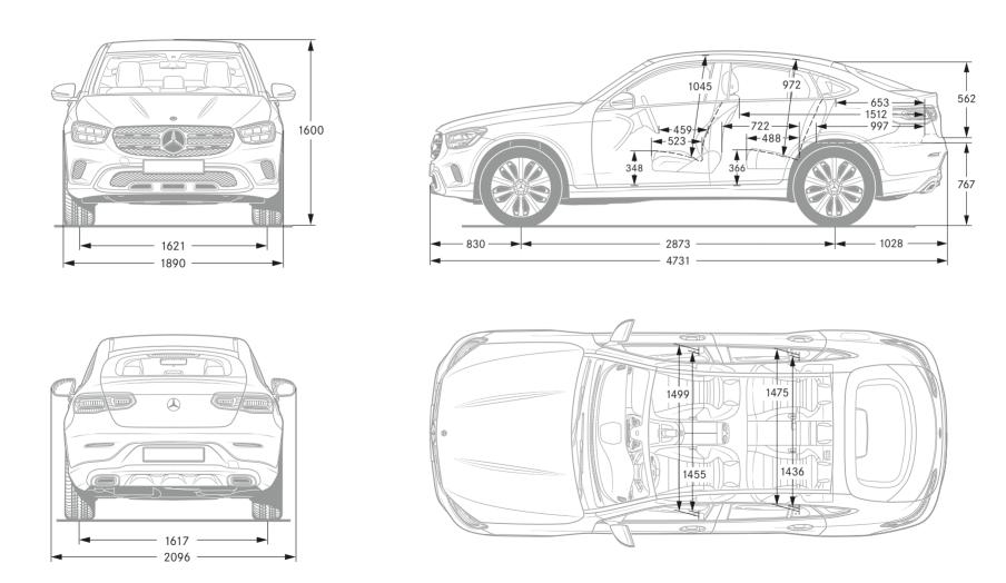
All figures in millimetres. The pictured dimensions are mean values. They are valid for vehicles in basic specification and in unladen condition.
